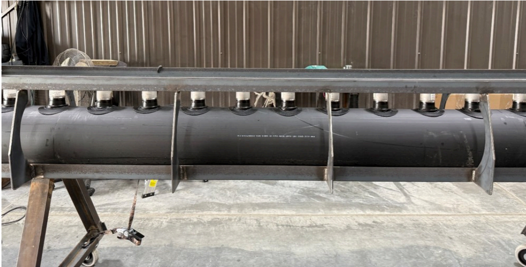
Photo 2. Construction of 10-inch manifold to accommodate the expected high flow rate at Shirley Basin
